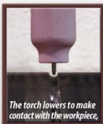
the tungsten preheats for an adjustable time...
