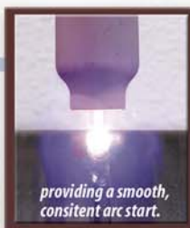
the tungsten preheats for an adjustable time...
